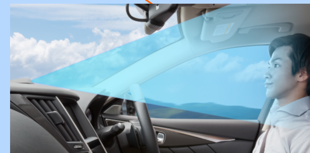
Driver monitoring system continually confirms the driver's attention is on the road
