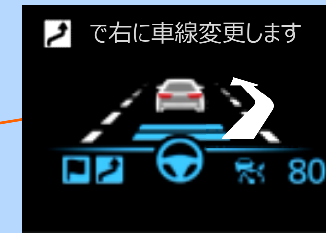
System suggests lane change timing by using map data and traffic conditions. Lane change assistance is initiated when the driver approves by pushing a switch
