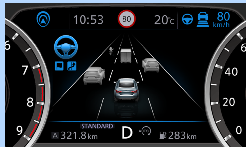
360-degree sensing information is displayed in real time
