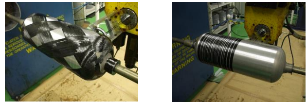
(a) Helical layer ( \pm 30^\circ degree). (b) Hoop layer.
