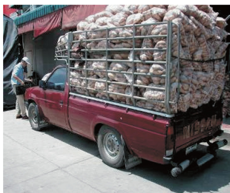
図-2 過積載での運搬 Fig. 2 Overloaded condition
