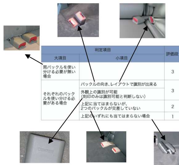
図-14 バックル識別性の評価方法 Fig. 14 Evaluation method of identification performance of seat belt buckle
