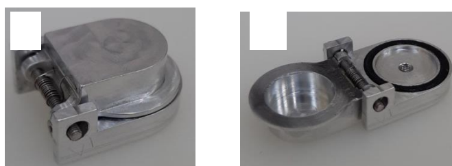
Figure 12. (a) Closed and (b) opened transfer chamber for SIMS and SEM analysis
