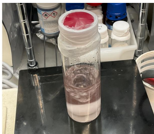
Fig. 8 Photo image of prepared electrolyte (LiClO 4 +EC DEC 3:7 v/v + 5m M Li 3 N)
