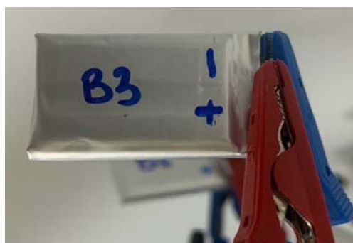
Figure 3. Photograph of the pouch cell used for cycling
