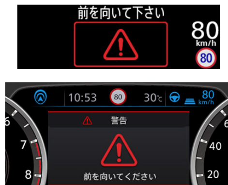
Fig.5 Driver-monitoring system and its warning for the driver to attend to the road ahead
