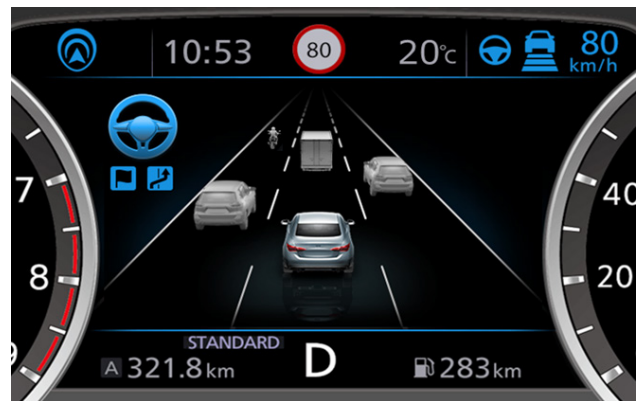
Fig.4 360° real-time surrounding display
