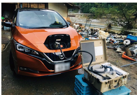
Fig. 3 Electricity supplied from Nissan LEAF
