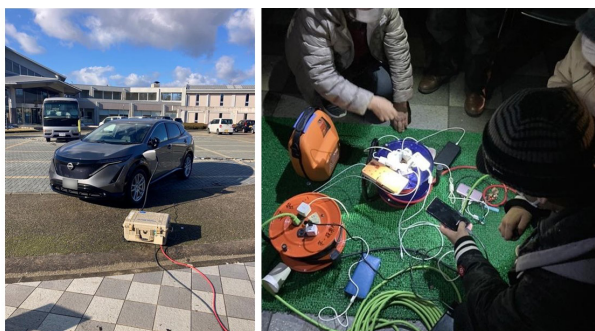
Fig. 4 Electricity being supplied from Nissan ARIYA
