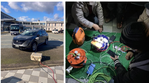
Fig. 4 Electricity being supplied from Nissan ARIYA
