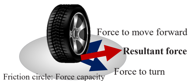
Fig.3 Tire friction circle and resultant force
