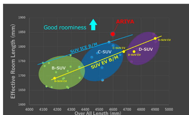
Fig.1 Comparison of overall vehicle and effective interior lengths between SUVs
