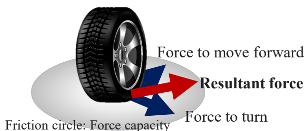
Fig.3 Tire friction circle and resultant force
