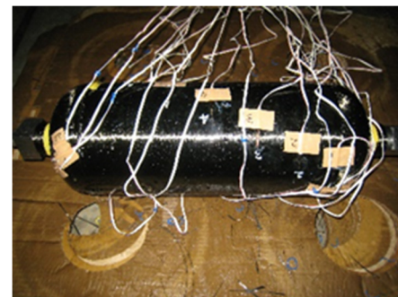
Fig. 5 Strain gauges on tank No. 4 set up.
