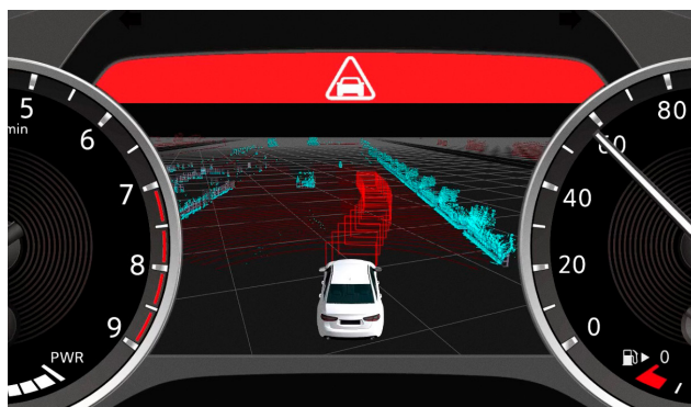
Fig. 8 Detection and avoidance of an approaching tire
