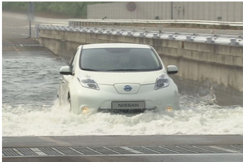
Fig. 9 Flooded road driving test
