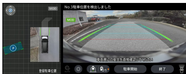
Fig. 7 Display when a parking location is automatically detected
