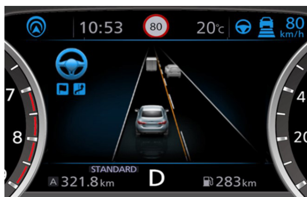
Fig. 15 Example of 360° real-time surrounding display (distinguishing line markings)
