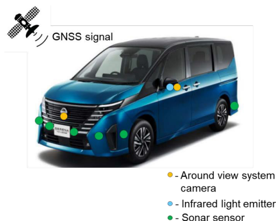
Fig. 4 Arrangement of the components of ProPILOT Park with memory function
