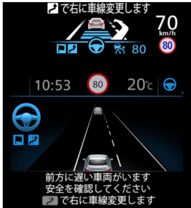
Fig. 13 Suggestions from the lane-change assistance system
