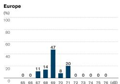
Noise emissions are shown by the noise produced by the acceleration of vehicle in accordance with each national regulation. Only complete, built-up imported models are shown for China data.
