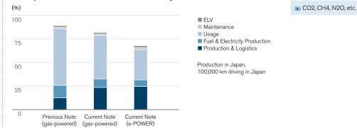
CO<sub>2</sub> Equivalent Emissions >> over Vehicle Lifecycle for Note e-POWER
