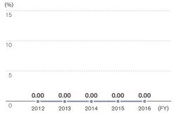
Based on the Automobile Recycling Law in Japan, Nissan calculated the ratio of landfill to residue after removing ferrous and nonferrous metals from ELVs. Nissan achieved a zero landfill ratio in fiscal 2016 by enhancing recycling capability through the acquisition of additional facilities that comply with the law.
