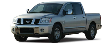
The Titan pickup sold in North America can run on fuel mixtures of up to 85% biofuel (E85).
