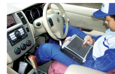
The Consult-III system allows accurate diagnosis of problems in today's complex cars. (Japan)
