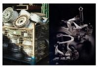
Suspension parts recycled from aluminum wheels
