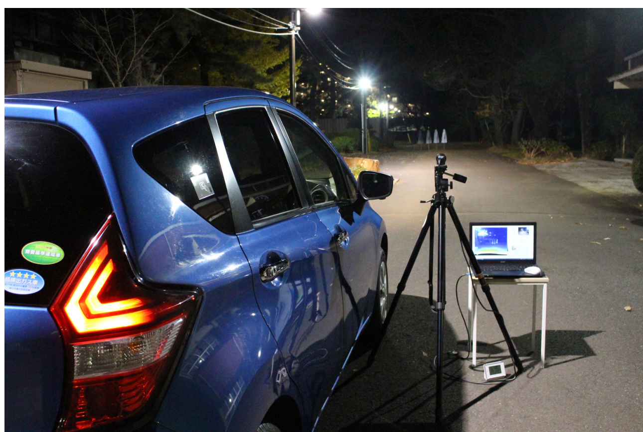
Experiment on the visibility of clothing in an outdoor setting (luminance measurement)
