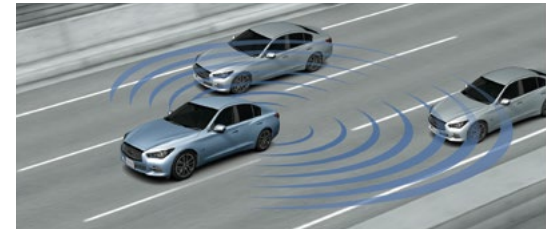
Blind Spot Warning and Blind Spot Intervention.
