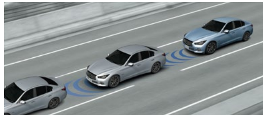
Predictive Forward Collision Warning.
