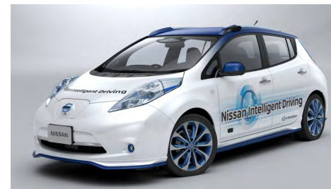
A Nissan Autonomous Drive test vehicle.
