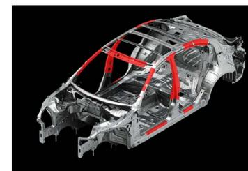
1.2 GPa Ultra High Tensile Strength Steel with High Formability in the Infiniti Q50 (red shaded areas)
