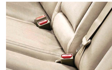
Self-standing buckles make seatbelt use easier for passengers in the rear seats.
