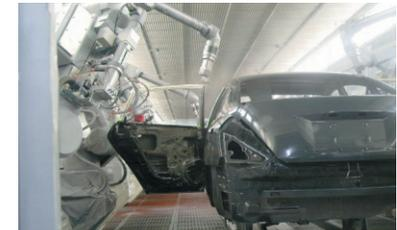
A Kyushu Plant line switched to water-based paint, producing less VOCs. (Japan)
