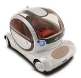
There's no need to go into reverse when entering or leaving a parking space. Drive the Pivo straight in, and when it's time to leave, rotate the cabin 180 degrees and drive straight back out.
