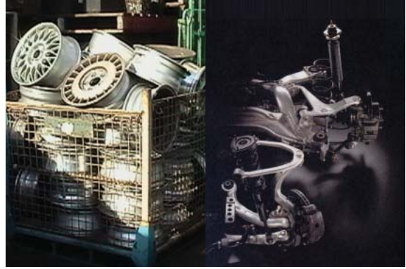
Suspension parts recycled from aluminum wheels
