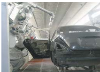
A line switched to water-based paint, producing less VOCs (Kyushu plant)
