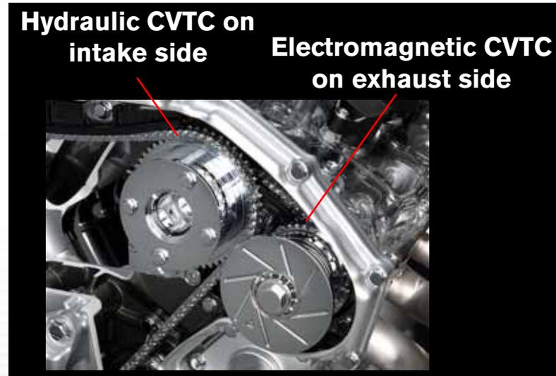
**CVTC intake and exhaust controls on both sides**
