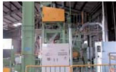
Recycling floor scraps with sorting machines (sorting wastes into steel, non-ferrous metals, sand or combustibles).
