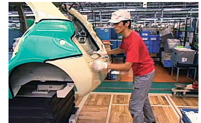
Workers had to squat to assemble parts before introduction of the "strike zone" approach (above); these stressful positions are no longer needed thanks to conveyors that can raise and lower the cars being worked on (below).
