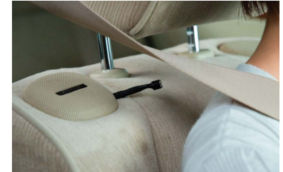
The driver's seat features an alcohol odor detection device.
