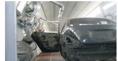
A Kyushu Plant line switched to water-based paint, producing less VOCs. (Japan)
