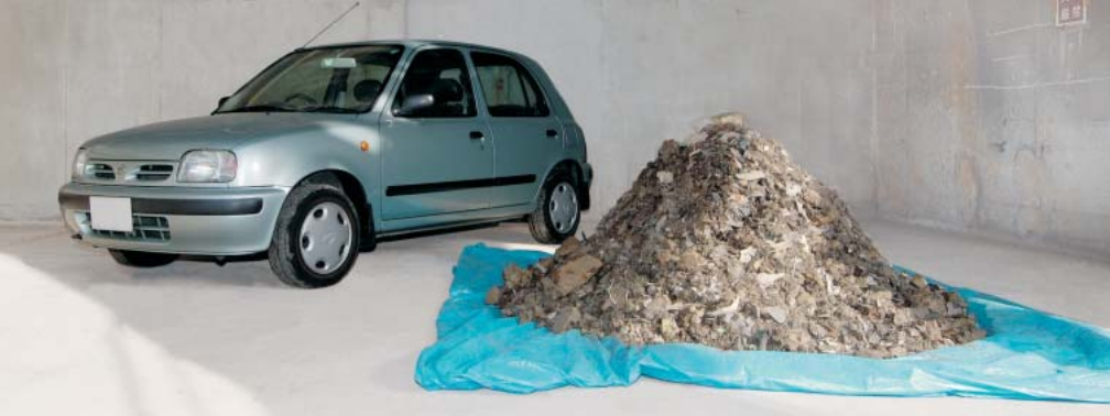
About 160 kilograms of ASR is generated from a single March vehicle (previous model).
