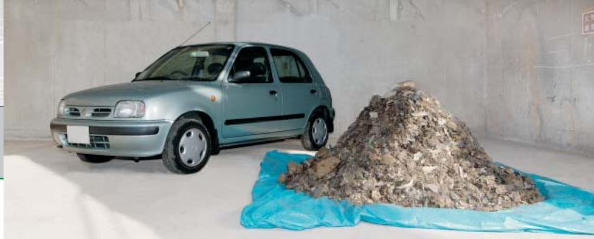
The amount of ASR generated from a single March vehicle (previous model)
