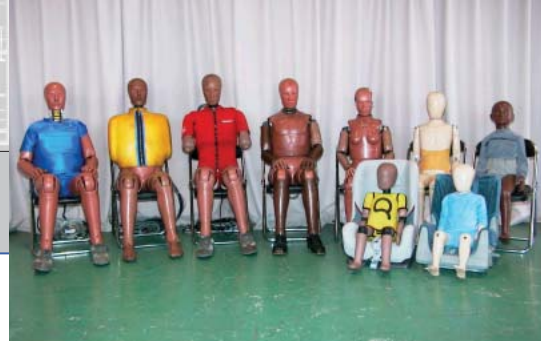
Specially designed dummies are used to confirm the safety performances of vehicles
