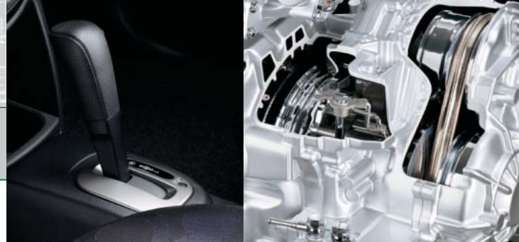
CVT (Continuously Variable Transmission) enables a smooth, continuous transmission which not only enhances acceleration, but which also improves fuel economy for better environmental performance
