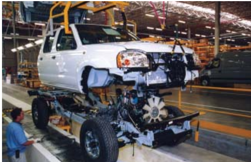
Production of the Frontier Pickup at Renault-Nissan common plant in Brazil
