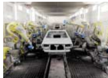
Adoption of water-based paints has reduced volatile organic compounds (VOC) at the Tochigi Plant, Japan.
