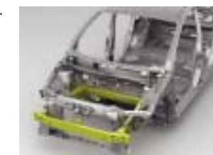
Crash-compatible Zone Body construction (Note)
