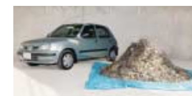
The amount of Automobile Shredder Residue (ASR) from a single vehicle of "March (previous model)".
