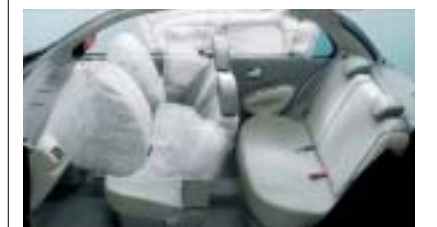
The SRS curtain airbag safety restraint system will be installed on virtually all Nissan passenger cars and RVs by FY2005.
