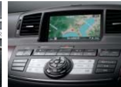
With a simple voice command, CARWINGS provides the latest traffic information, e-mail functions and many useful information for driving.
