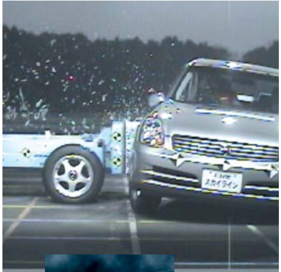
A collision test for Skyline (Top), a Nissan model that was given the highest, six-star rating for overall collision safety performance in the FY2001 New Car Assessment Japan*.
