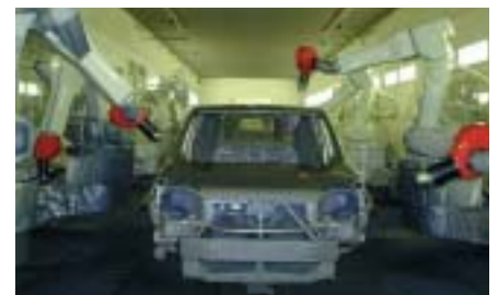
Adoption of water-based paints has reduced volatile organic compounds (VOC) at the Kyushu Plant, Japan.
