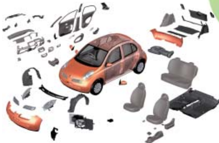
The new March achieves a 95 percent recyclability rate. (This mass-based figure is calculated with Nissan's in-house standard)
