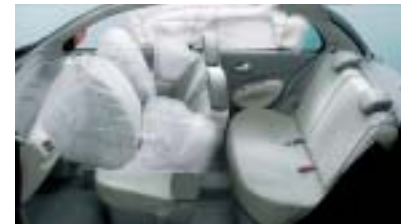
The SRS curtain airbag safety restraint system will be installed on virtually all Nissan passenger cars and RVs by FY2005.
