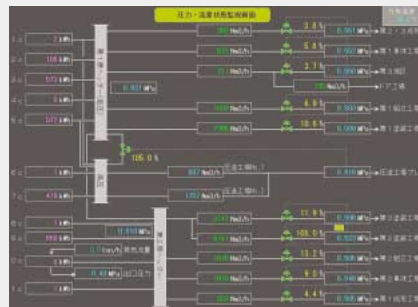
The compressed air supply device drive's control panel
