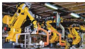
Body welding equipment
