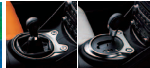
Synchronized Rev Control (6MT) and 7-speed Automatic Transmission
