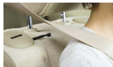
Passenger seat alcohol odor sensor in the anti drink—driving concept car
